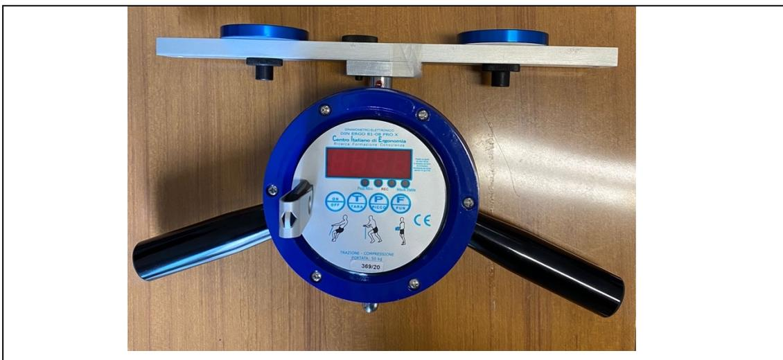
Figura 6: dinamometro DIN ERGO 81-08 PRO-X
